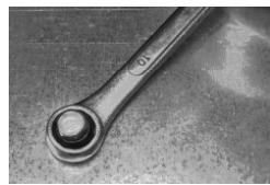
Holding the M6 hex nut firmly with a 10mm wrench , tighten the hex bolt with a 8mm wrench until the Plus nut insert collapses (there will be a noticeable force increase).
