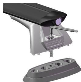
Re-Install cross bars onto adapter bases and tighten anchor point screws firmly into adapter nuts
