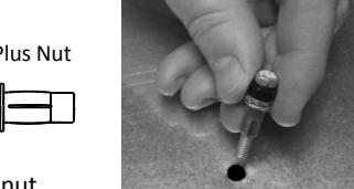
Install Plus Nut inserts into drilled holes.
