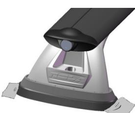
Once aligned correctly tape adapters to surface. Carefully remove cross bars.
