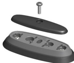
Install covers when cross bars are not installed to keep debris out of adapters
